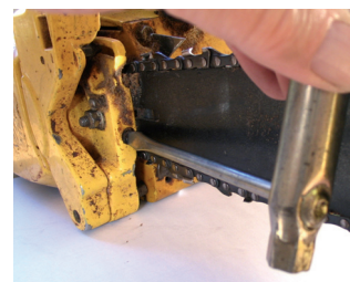
Tensioner screw on a McCulloch chainsaw
