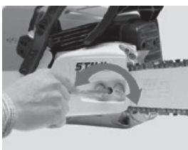
Tensioner screw on a Stihl chainsaw
