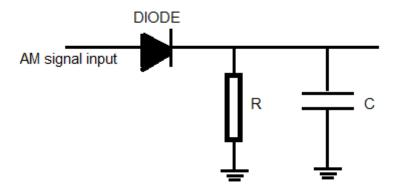
FIGURE 14.2: DIODE DETECTOR CIRCUIT WITH CAPACITOR
