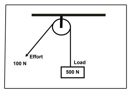
Calculate the mechanical advantage.
