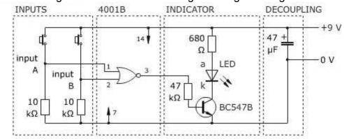
The inputs of the gate *must* be connected, either to LOW or to HIGH, and *must not* be left open circuit. This is the function of the input switches with their pulldown resistors. To avoid loading the output of the gate, a transistor switch indicator circuit should be used.
