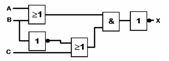
**3.** Draw the logic gate circuit for the Boolean Equation  $X = \overline{(A+B)} \overline{C}$ (4)
