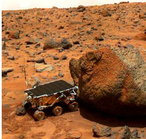
This is the rover that was carried by the Pathfinder spacecraft. It has instruments to find out what the rock is made of.
