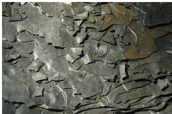
Shale splits easily into thin tiles which can be used in flooring and roofs.
