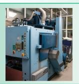
During the spinning process, the wool is stretched and plaited.
